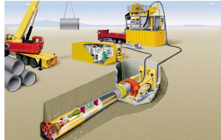
Microtunnelling launch shaft
